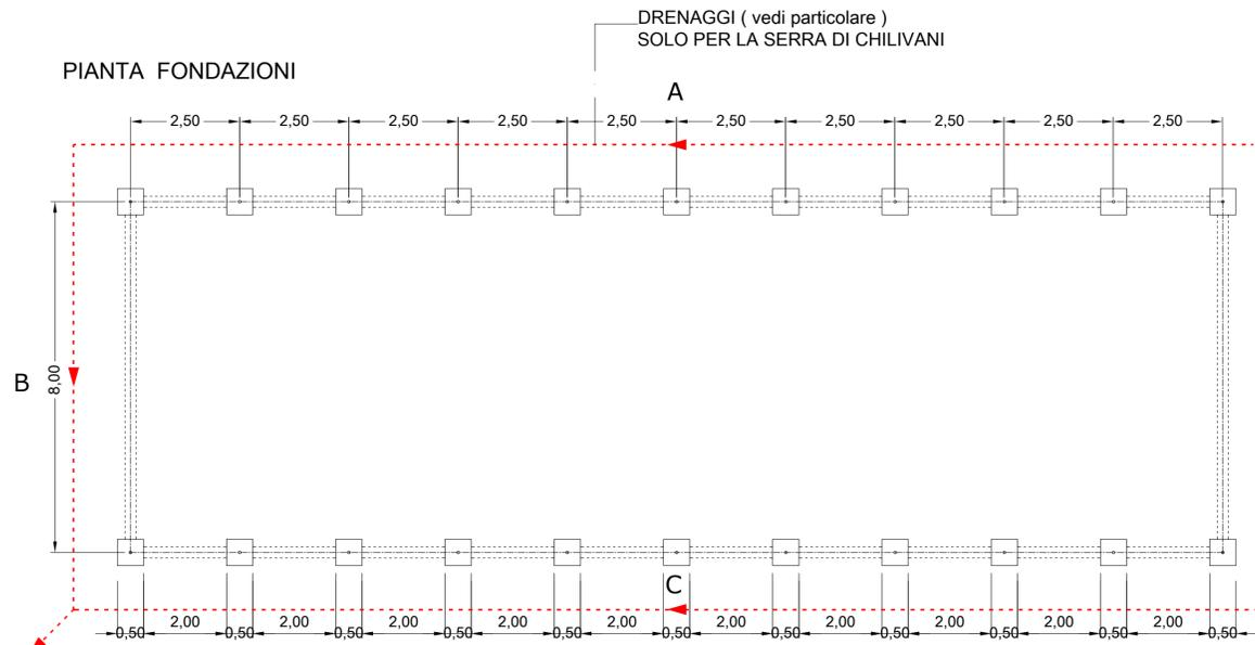
IL PRODUTTORE DELLA SERRA PUO' PREVEDERE IN ALTERNATIVA AI PLINTI APPOSITE ANCORE A VITE IN ACCIAIO ZINCATO PER OGNI TUBO TONDO VERSO TERRA, CON SISTEMA CERTIFICATO E APPROVATO DALLA D. L.
